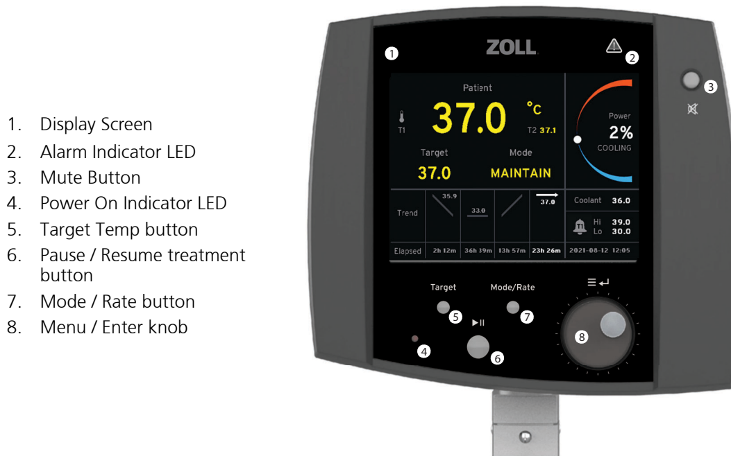
Figure 2.2. Controls and Display Screen
